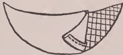
Fig. (140) The facing slipped over the foundation peak
